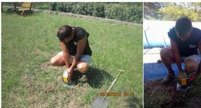
Photo 1 : Mesures pXRF (NITON®)
